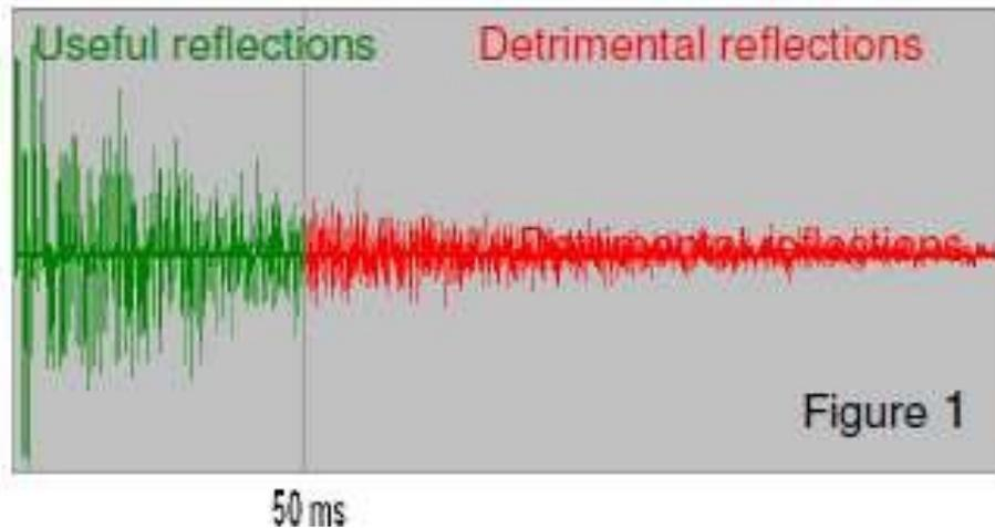
$$C_{50} = 10 \log_{10} \frac{\text{Energie}(0 - 50 \text{ ms})}{\text{Energie}(50 \text{ ms} - \text{fin})}$$
